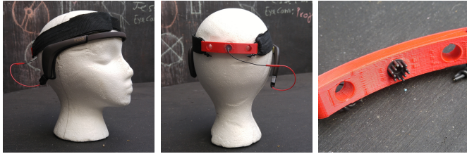
Fig. 4. Left: Side view of Muse 2. Middle: Rear view of Muse 2 and custom electrode band. Right: Front view of custom electrode band.
